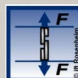
Tensile shear strengths of >10 N/mm<sup>2</sup> at 80 °C are being achieved in heat resistance tests according to the testing instruction EN 14257 (Watt 91). The recommended minimum strength for the manufacture of window scantlings is just >7 N/mm<sup>2</sup>. The tensile shear strengths required for durability class D4 (according to EN 204/205) are also being exceeded significantly by these adhesive systems.
